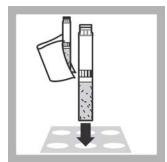
7. Clean the vial. Insert the vial in the preheated DRB200 reactor. Close the lid. Keep the vial in the reactor for 10 minutes.
