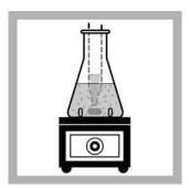
2. Stir the sample in a baffled flask with a magnetic stir plate.
