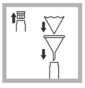
**10.** Remove the cap from the TNT882 vial. Put the filter paper in the funnel. Insert the funnel in the TNT882 vial.
