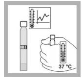
**11.** If there is a small amount of turbidity in the chloroform phase, increase the temperature of the vial (e.g., hold the vial in a hand).
