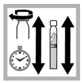
**7.** Put the cap on the vial. Hold the vial by the cap. Carefully shake the vial for 2 minutes.
