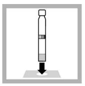
**14.** Put the vial into the cell holder. DR 1900 only: Push **READ 2**. Results show in mg/L cetyltrimethylammonium bromide.
