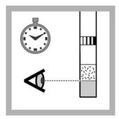
**8.** Keep the vial vertical for 30 seconds to let phase separation occur.
