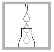
**4.** Use a pipet to add 4.0 mL of sample to the vial.
