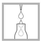
**5.** Use a pipet to add 0.4 mL of Solution A to the vial.
