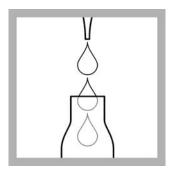
**6.** Use a pipet to add 0.2 mL of Solution B to the vial.
