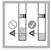
**10.** If streaks or small drops of water form in the lower part of the vial, carefully tilt the vial 90 degrees and rotate the vial.
