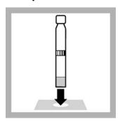
1. Put the vial into the cell holder. DR1900 only: Select program TNT885. Push READ 1. Refer to Before starting on page 1.
