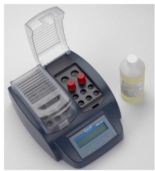
minimizing sample exposure, as does the use of a combined sampling-digestion vial. The sample is taken directly into the DRB200 digestion vial. FerroZine reagent is added. The vial is capped and digested. The digested sample is sipped or poured into the sample cell and read. With careful technique, a simple, inexpensive, and timely ULR total iron determination can be performed in the typical power plant laboratory.
