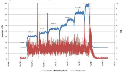
below 0.5, is indicative of a particle-free baseline, and anything above this value is indicative of the presence of particles.<sup>(12)</sup> The RSD value is a confirmative response to the elevated turbidity values that result from the particulate iron. The RSD parameter may be used as a leading indicator of iron transport as it is sensitive to the leading edge of any slug transport.
