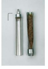
5. After locating the intended spot, press the auger vertically into the ground to the desired depth. If necessary an impact absorbing hammer can be used to drive the auger into the ground.
