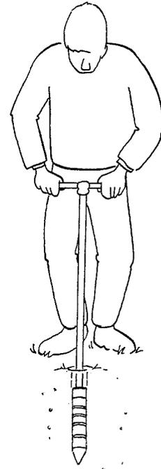
3. Insert the EC-probe vertically, and without rotating it, into the pre-augered borehole (see figure). To obtain optimum results the probe should be in full contact with the soil. For immediate temperature adjustment, the probe's cone should well touch the soil.
