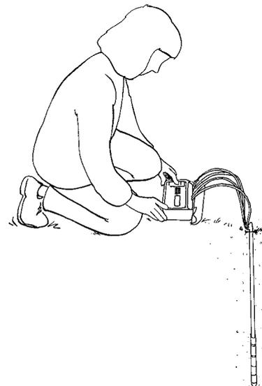
6. Start measuring. Push the "Test" (measure) button of the earth resistivity meter, hold it down until the measuring value shows on the display. Check the failure indicators again. If necessary, correct the situation and repeat measuring. Upon releasing the button, the instrument switches off immediately. Take down the measured resistivity. This will be the measured resistivity at the prevailing temperature:  $R_t(\Omega)$ .
