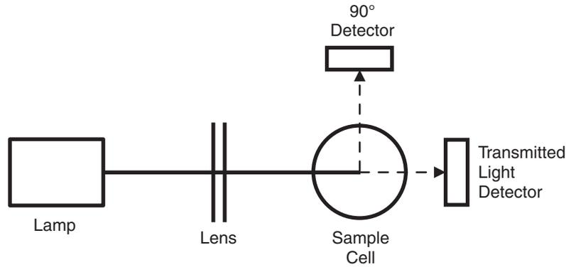
Figure 4 General turbidimeter optical system
