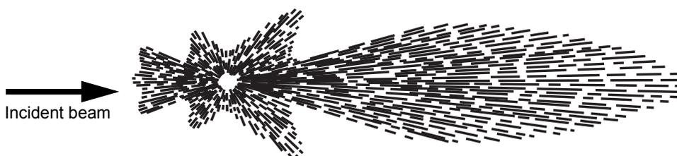
Figure 3 Effects of particle size and light wavelength (larger particles)<sup>1</sup>
