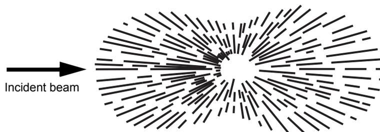
Figure 1 Effects of particle size and light wavelength (small particles)<sup>1</sup>
