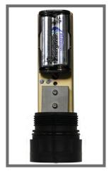
The miniDOT Clear Logger is a completely submersible instrument that logs dissolved oxygen and temperature measurements and has an internal LCD screen, which displays real-time measurements. The oxygen sensor is an optode that measures dissolved oxygen concentration in water through a fluorescence method. Data are recorded to an internal SD card. Operation of the miniDOT Clear Logger such as setting the time and sample interval can be accomplished via the USB cable.
