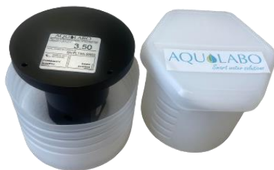
Figure 2 : Signal control tool with specific box for safe storage
