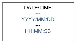
To change the date and time place the cursor on the desired line and use the Up/Down arrows to change the numbers from 0 to 9. The writing then changes to white. Confirm your setting with the OK key (the writing changes to green). To return to the previous screen, press the Escape (ESC) key.
