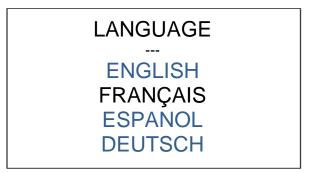
To select the language, use the Up/Down arrows (writing changes to white) and confirm using the OK key. To return to the previous screen press the Escape (ESC) key.
