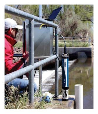
The HYDROLAB HL7 multiparameter sonde offers a versatile, durable and practical solution to the day to day needs of monitoring programs for both simple and complex deployments. The HL7 sonde, with a large sensor suite, is able to thrive in demanding environmental conditions for long term continuous monitoring.
